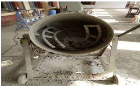
Figure 2 Drum type mixer
