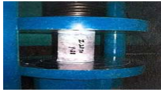
Fig. 7 After dressing the concrete core specimen kept in the compressive testing machine for compression test
