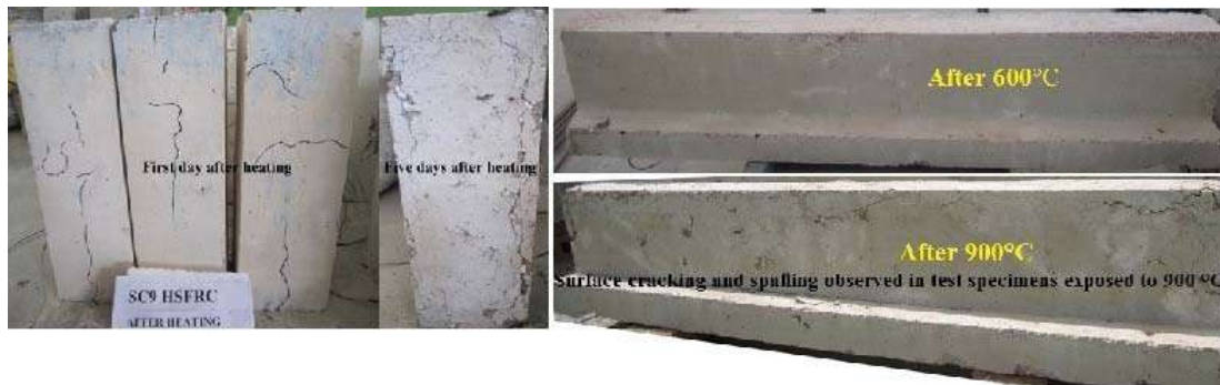
Fig. 3 Surface cracking observed in test specimens exposed to 900 °C
