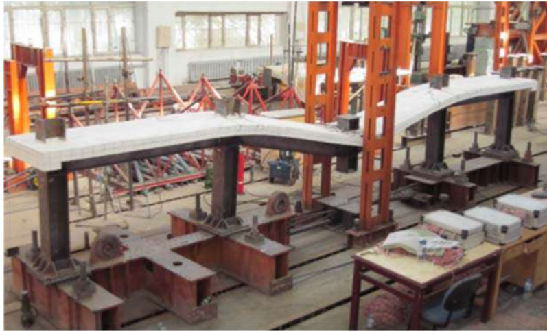
Fig. 2. View of a test by Guo et al. on a composite frame. Photo by courtesy of Lanhui Guo (Harbin Institute of Technology).
