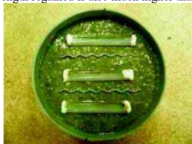
Fig.5.Specimens with glass tubes filled with polyurethane as healing agent
