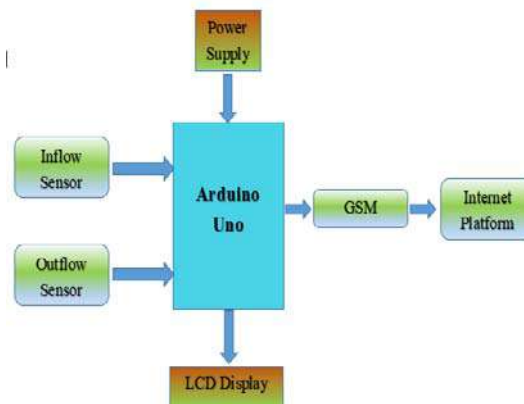
Fig. 3 Block diagram of water leakage monitoring system
