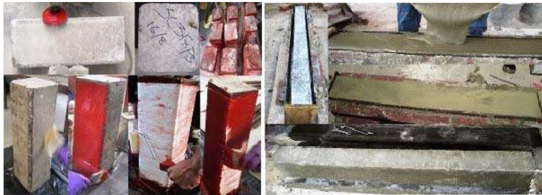
Fig. 4 Strengthening process of GFRP jacketing and HSFRC jacketing
