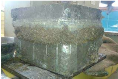
Figure 2: Model showing rice husk layer as a sub base
