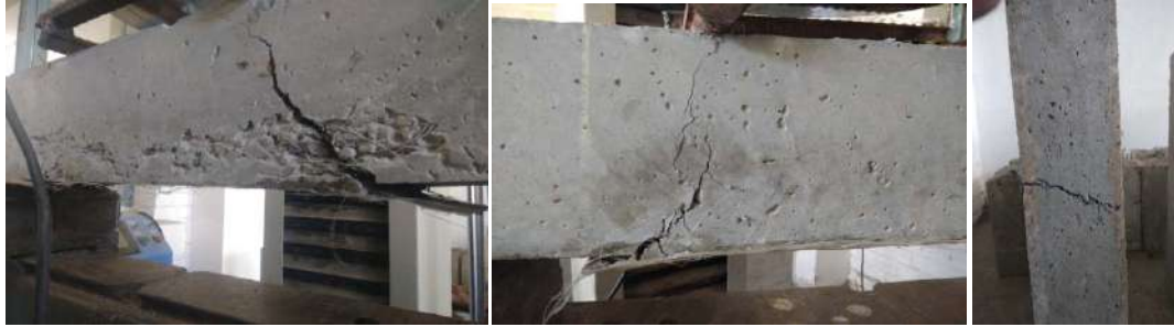
Fig. 2 Diagonal Cracks depicting shear failure
