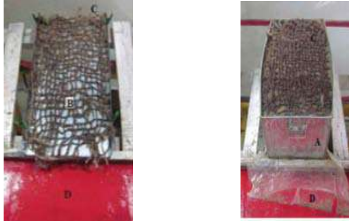
Fig. 2 Sample placement for testing in soil infiltration and zero infiltration condition
